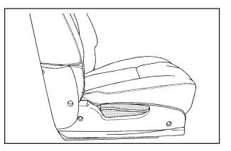
To recline the seatback on the front passenger's seat, lift the lever, located on the outboard side of the seat, up fully to disengage the seatback. Then move the seatback to the desired position. Release the lever to lock the seatback in place.
